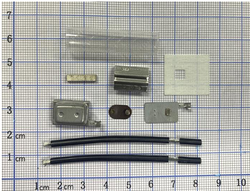
Model ST07016A5PTC, ST07043A5PTC internal structure diagram
